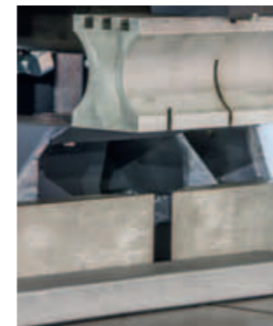
Work piece stop and clamping on both sides of the saw blade.
