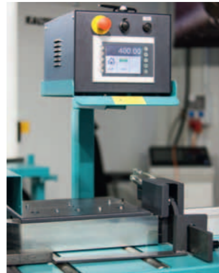
Universal mitre circular saw with length measurement system L 41 NC and T3 infeed conveyor system.
